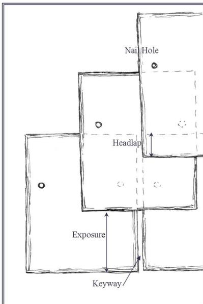
To understand how a slate roof works you first need to know the parts and terms
