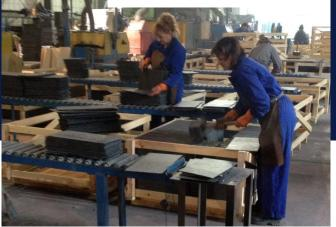
Before the slate is sent out each slate is "sounded" (sounding— tapping each slate for a solid ring, slate with a hairline fracture will not produce a solid ring sound).
