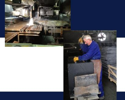
Each stone is cut down into square sections. Larger sections may be harder to split but they may also be cut down in size later.
