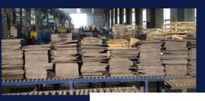
After being split into "chips" the slate is cut to size with the chamfered edges. The detail on the edges of slate will give the roof an unique look, synonymous to natural slate.
